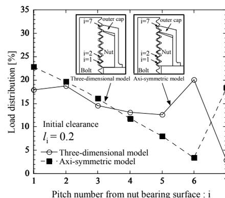
Fig. 7(b) Comparison between 3D and axi-symmetric models for load distribution of outer cap nut (SS400 outer cap,  $l_i=0.2\text{mm}$ ,  $\theta=105^\circ$ ,  $F_b=44.6\text{kN}$ )
