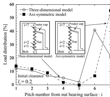
Fig. 7(a) Comparison between 3D and axi-symmetric models for load distribution of outer cap nut (Elastic outer cap,  $l_i=0.2\text{mm}$ ,  $\theta=105^\circ$ ,  $F_b=52.9\text{kN}$ )
