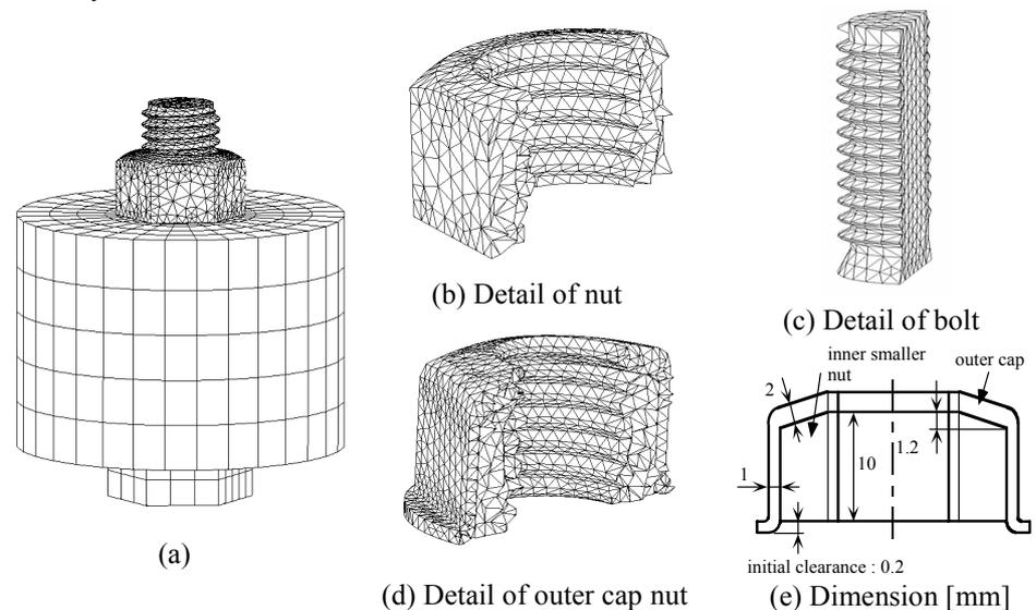
Fig. 5 Three-dimensional finite element model for bolted joint (a) (b) (c) and outer cap nut (d) (e)
