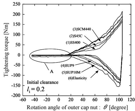
Fig. 15(a) Effect of material difference for tightening torque by three-dimensional model ( $l_i=0.2\text{mm}$ ,  $\theta=-45^\circ$ )
