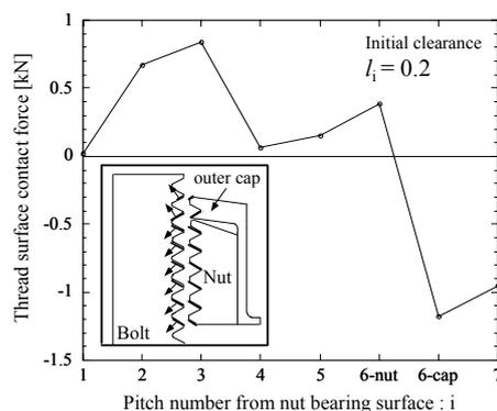
Fig. 14 Thread surface contact force by three-dimensional model (Elastic outer cap,  $l_i=0.2\text{mm}$ ,  $\theta=-45^\circ$ )
