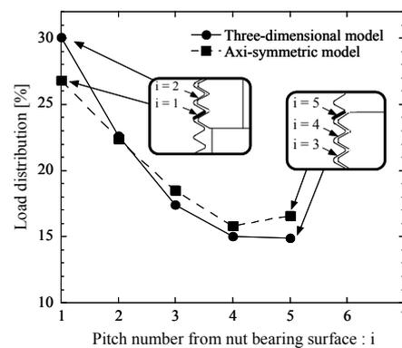
Fig. 6(b) Load distribution of bolt-axial force of standard nut (Comparison between axi-symmetric and 3D models)
