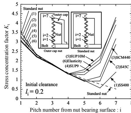
Fig. 11 Stress concentration factor of outer cap nut by axi-symmetric model ( $l_i = 0.2\text{mm}$ ,  $F_b = 44.6\text{kN} - 52.9\text{kN}$ )
