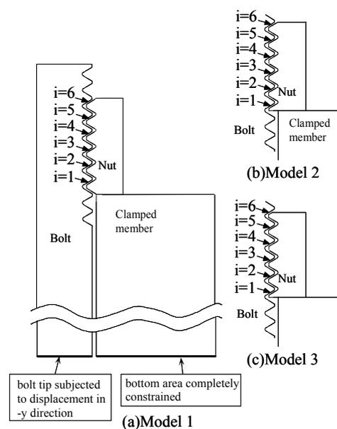
Fig. 3 Axi-symmetric bolted joint model
