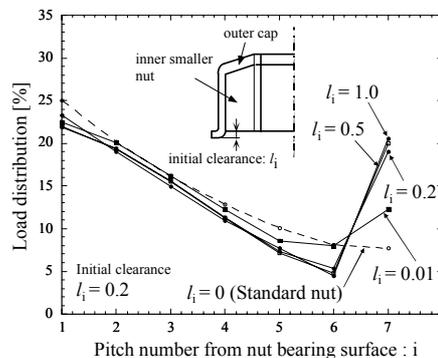
Fig. 10 Effect of initial clearance of outer cap nut by axi-symmetric model (SS400 outer cap,  $l_i=0.2\text{mm}$ ,  $F_b \approx 45\text{kN}$ )
