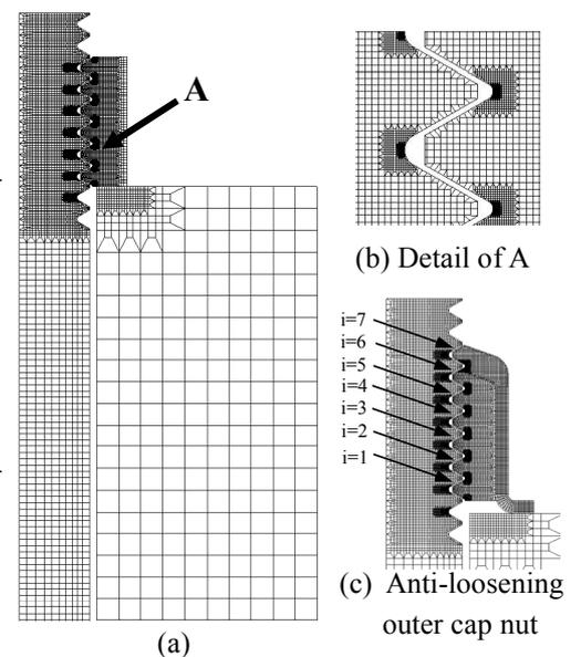
Fig. 4 Axi-symmetric finite element model for bolted joint
