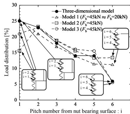
Fig.6(a) Load distribution of bolt-axial force of standard nut with incomplete threads at both ends
