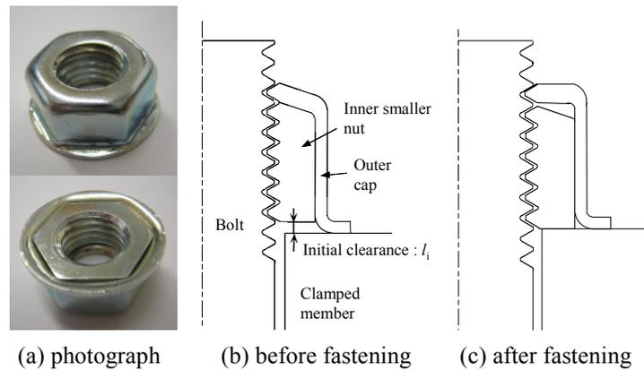
Fig. 1 Super Loose Proof (Anti-loosening outer cap nut)
