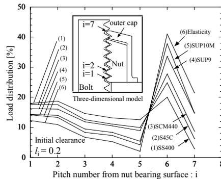
Fig. 9 Effect of material difference of outer cap nut by 3D model ( $l_i=0.2\text{mm}$ ,  $\theta=105^\circ$ ,  $F_b=44.6\text{kN}-52.9\text{kN}$ )
