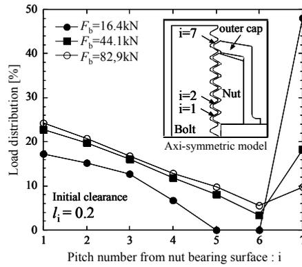
Fig. 8 Effect of bolt-axial force  $F_b$  by axi-symmetric model (SS400 outer cap,  $l_i=0.2\text{mm}$ )
