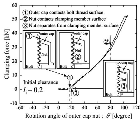
Fig. 12 Relation between clamping force and rotation angle of outer cap nut by three-dimensional model (Elastic outer cap,  $l_i = 0.2\text{mm}$ )
