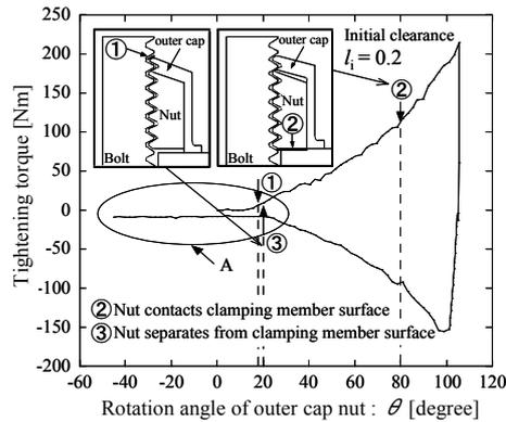
Fig. 13(a) Relation between tightening torque and rotation angle of outer cap nut by three-dimensional model (Elastic outer cap,  $l_i=0.2\text{mm}$ )
